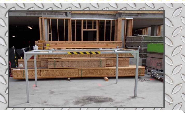
The Aerial Frame is built of heavy-duty galvanized steel and disassembles quickly into 4 pieces for easy transport.
