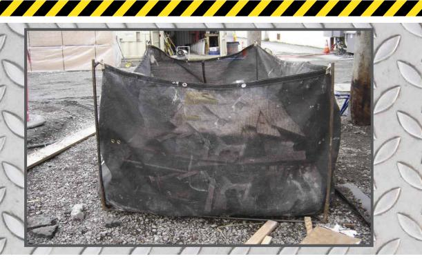
The lightweight, high strength mesh Cranetainer can be lifted to any solid surface a crane or forklift can reach, without damaging that surface.
