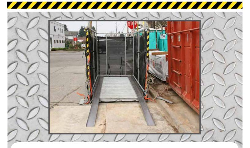
The Track System is a set of metal tracks with ramps that allow filled Material Racks to be quickly rolled in and out of the Material Handler. Using multiple Material Racks creates a continuous flow of loading and unloading when large quantities of like materials need to be moved.
