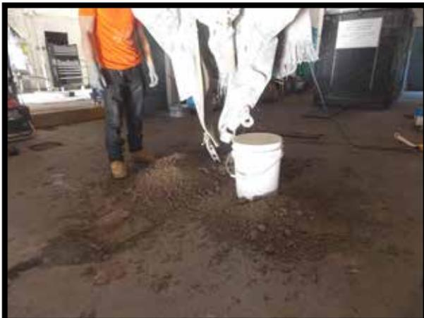
Do not use Cranetainers as a wash out area for slurry from pump equipment. This action pushes the silt material in between the layers of the Cranetainer. If this happens, the Cranetainer has to be cut open to remove the material. This increases cleaning and repair costs.
