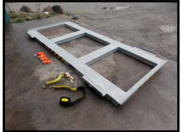
**The Stabilizing Straps are there only for the purpose of stabilizing the Material Handler when driven over rough terrain or curbs. DO NOT EVER LIFT THE MATERIAL HANDLER FROM THE FOUR-WAYS (with a crane or forklift) WITH THE FORKLIFT RACK ATTACHED TO THE MATERIAL HANDLER BY THE STABILIZING STRAPS.**
