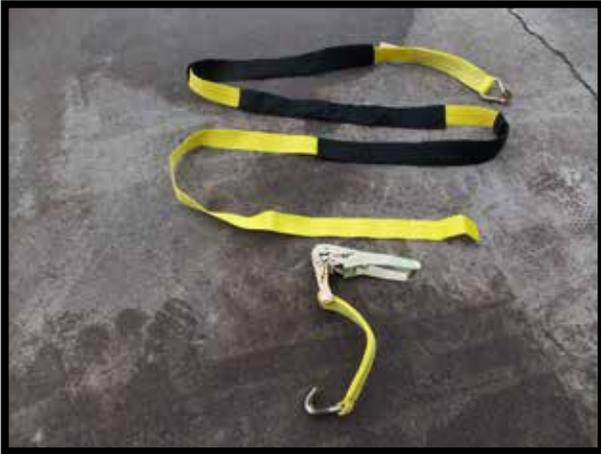
The Forklift Ratchet Tie Down is comprised of two components: a ratchet end and a tail end. The tail end has three black Fabric Guards that need to be slid into place on the sharp edges of the forklift cage.
