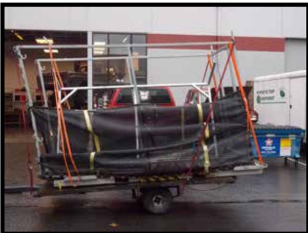
All components and accessories are necessary for the proper operation of the equipment. This Material Handler was operated without a Ratchet Tie Down Strap and due to operator error was dropped from 20 feet in the air. It landed on the concrete causing severe damage to the Material Handler.
