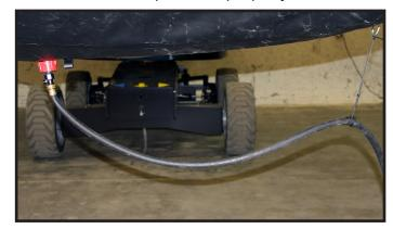
Spilled liquids can be drained at floor level using the valve at the bottom of the Lift Pan. Workers can also attach a hose to the Lift Pan to drain or remove liquids from overhead equipment.
