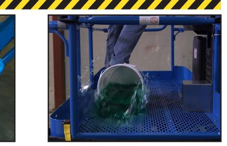
Spilled liquids can cause costly damage and possible injury to people or objects below. If materials are spilled, the Lift Pan is able to safely contain them so they can be recaptured or disposed of properly.
