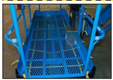
The unique tensioning system prevents the Lift Pan from being blown off by wind or other physical contact.
