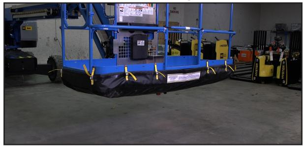
The Lift Pan is designed for spill containment of liquids and dry materials from within the Lift basket work area. It is made of a high strength vinyl covered polyester grid and has windows to aid visibility. The Lift Pan has a maximum working capacity of 15 gallons.
