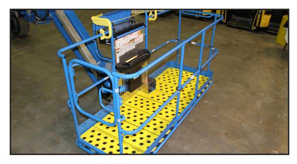
The Lift Screenmat gives workers a comfortable, ergonomic working surface. The Lift Screenmat is made up of two layers of durable closed cell foam with a layer of high strength mesh in between. The mesh barrier catches all small objects, preventing them from falling through the basket and causing a safety hazard or equipment damage below.
